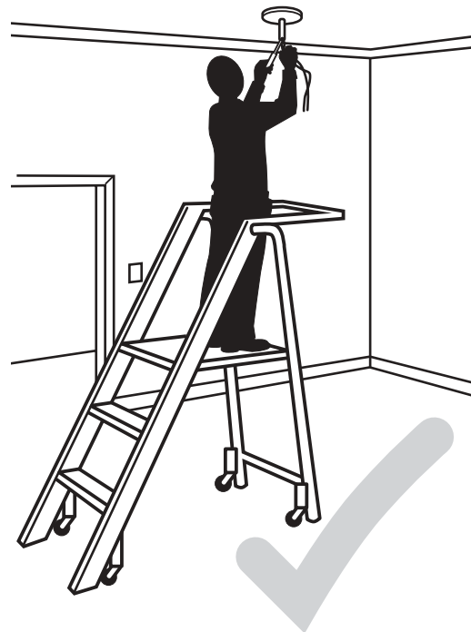
Above: A step platform can provide a stable work surface.
